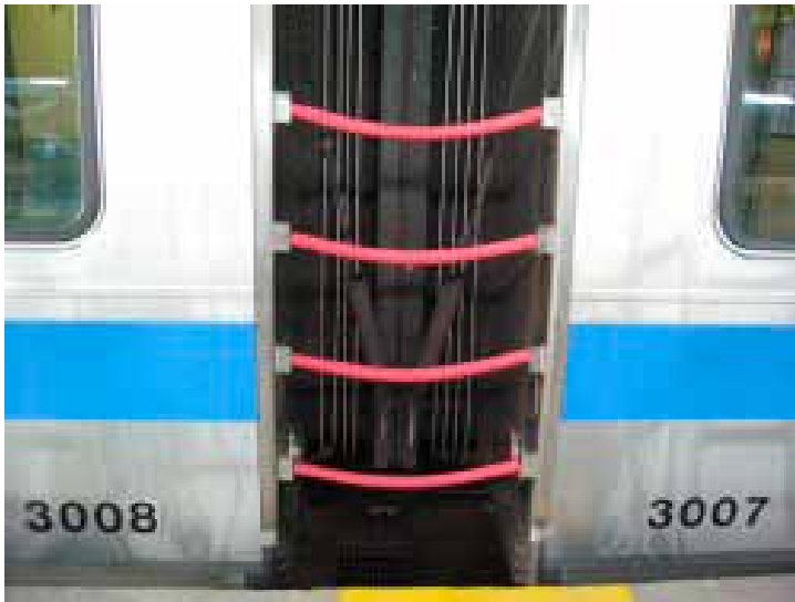
Fall Prevention Barrier– for safety of vision impaired travellers moving between carriages.
